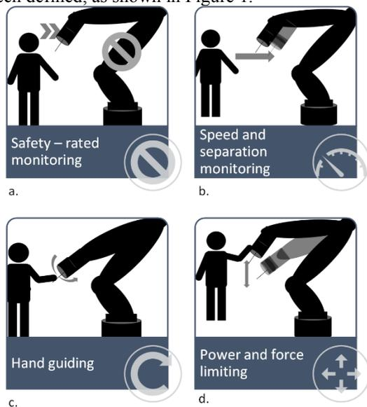
Figure 1. (a) Robot stops when operator enters the collaborative area; (b) Contact is prevented; (c) The operator controls the robot movements actively; (d) Contact forces are limited.
