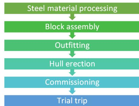
Figure 2. Six main stages of shipbuilding
