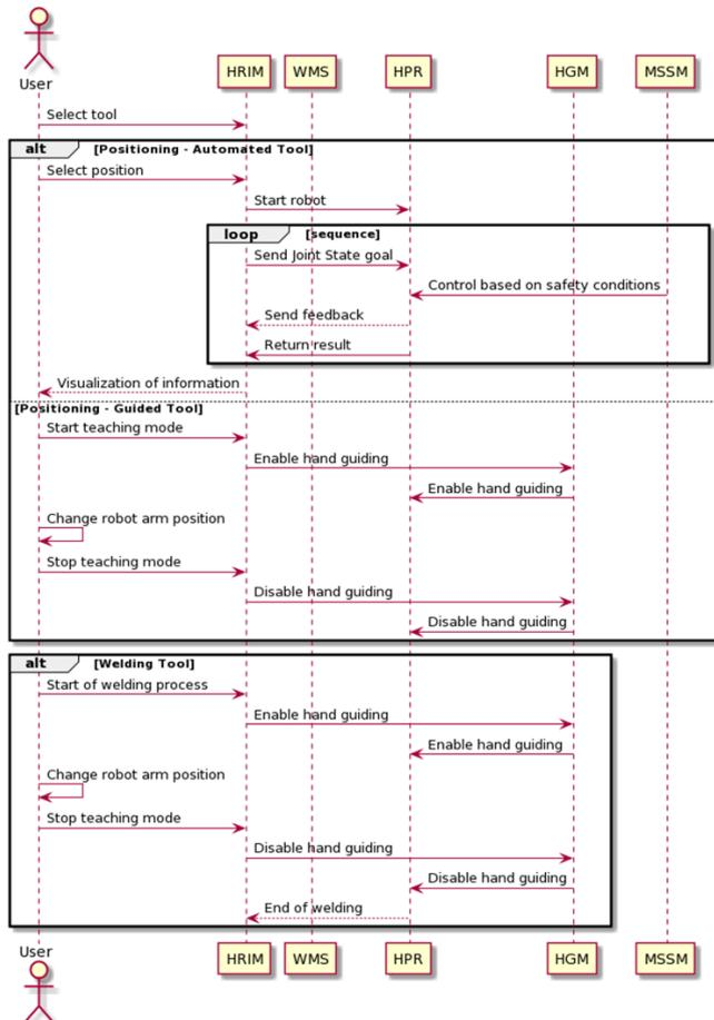
Figure 6. UML diagram demonstrating the communication between the modules applied in this use case
