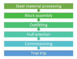
Figure 2. Six main stages of shipbuilding
