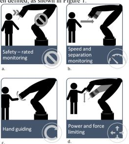
Figure 1. (a) Robot stops when operator enters the collaborative area; (b)
