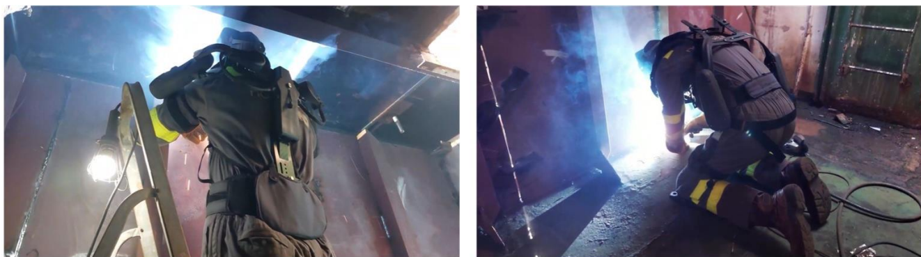
Figure 6. Wearable robotics. Exoskeletons supporting operator in welding activities.
